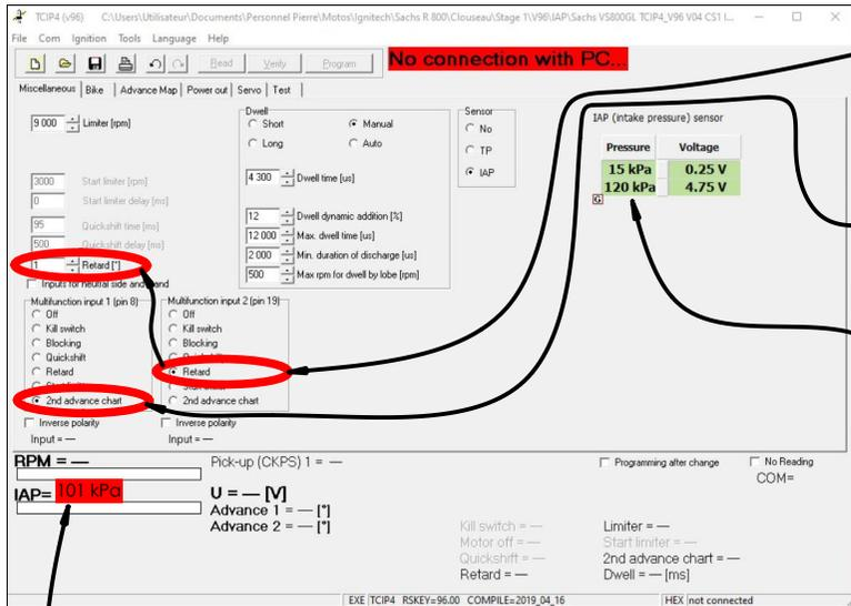
Retard: -1°. A security to reduce the programmed values with an optional connector from "pin19" to "ground".
